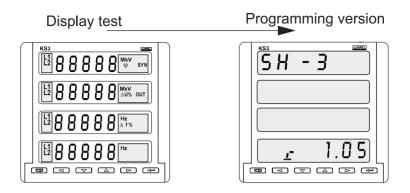
This sequence appears after each start of the instrument. The measurement mode starts after carrying out the tests.
