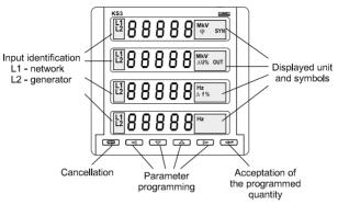
Fig. 3. View of the KS3-1 unit frontal plate
