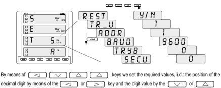
key. The cursor signals the active position. The value is accepted by the Common key, after pressing we set
