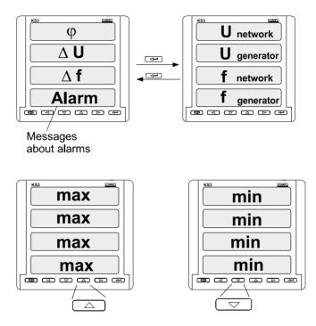
Displaying of minimal and maximal values.
